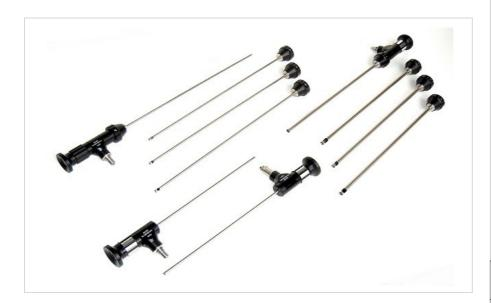
Borescopes with rotatable mirror tubes are versatile inspection instruments. This range enables 0°, 70°, 90° and 110° directions of view. A protection tube for 0° use is included as standard. The instruments use high quality rod lenses for the image surrounded by glass fibres for illumination.
